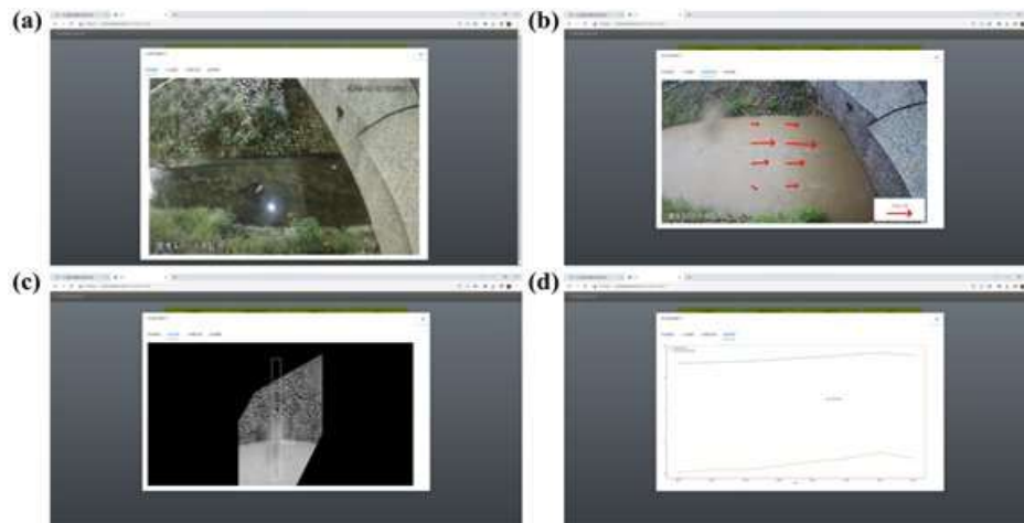
Figure 2. Web dashboard: (a) live imagery, (b) surface velocity field, (c) virtual water gauge, (d) discharge time series
